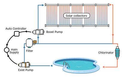
\* The booster pump is shown here installed after the filter. Alternatively, if separate solar lines have been installed into the pool, the solar system can ideally be installed on a separate circuit. Ask your Heliocol supplier for details
